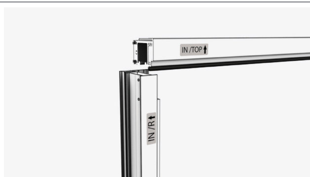
FIG. 1 Frame piece markings — Label side faces the interior
